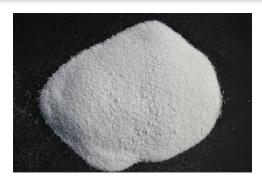
As the natural materails, Expanded Perlite and Clay are two candidates for building materials which comply nearly all features but having lack of strength problem.
