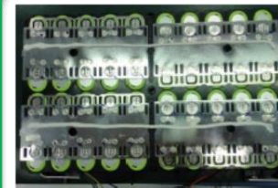
Housing mechanical, insulator, nickel plate design
